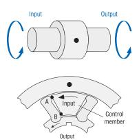
The control member projects between each pair of opposing sprags and when driving torque is applied to it, each projection first contacts a sprag at point "A" to disengage the sprag from the **outer race**. Then, the **control member** drives against the sprag at point "B" to transmit driving torque directly to the **output member**.
