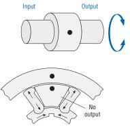
Any feedback torque from the **output member** is instantly stopped by the wedging of sprags between the fixed outer race and the **output member** feedback torque never reaches the **control member**.
